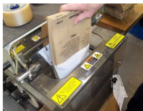
Hiretech print label information directly onto the bag using a 300dpi Autobag Precision printer
