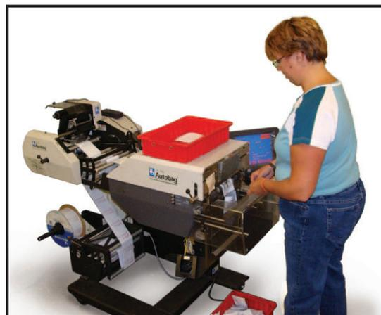
The Autobag AB 180 bagger is used as a semi-automatic system with one operator hand loading the product into a pre-opened bag that is automatically positioned for easy insertion and then automatically sealed and dropped into a bin for distribution. The bags are printed in-line with the proper barcode and product information, eliminating the need for a separate label. The Autobag AB 180 is capable of packaging up to 80 bags per minute and changeovers between jobs take less than two minutes.
