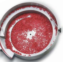
Stainless steel, as well as coated cast aluminum bowls, can be utilised with the AccuCount 200.
